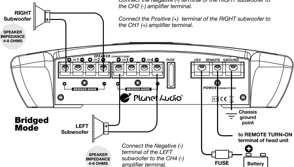
Connect the Negative (-) terminal of the LEFT subwoofer to the CH4 (-) amplifier terminal.
