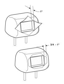
Set the adjustable blade to 1" depth, and cut around the edges of the hole, staying 1/4" inside the edge. Pull up one corner of the foam rectangle, and use the blade to cut underneath – remove a small section at a time, using the "pull up and cut" method for uniform depth. If necessary, use a Dremel tool or other appropriate tool to remove any other obstructions present.
