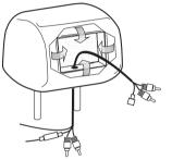
Route the cable through the opening just cut, and out the bottom of the headrest. If possible, conceal the cable using a gear shift covering or similar. Then fold the four flaps into the cavity in the headrest.
