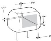
Using a sharp, adjustable-depth blade knife, make a diagonal cut beginning 1/4" INSIDE from one corner, and ending 1/4" INSIDE from the opposite corner.
