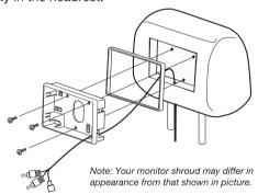
Slide the trim frame onto the monitor shroud and slide the assembly into the cavity in the headrest. As you do this, feed the cable through the headrest as shown in the diagram. Secure the shroud with the three screws as shown.
