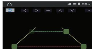
Touch and drag a square icon to reposition the related guide line. Repeatedly touch an arrow icon to fine tune positioning of the related guide line. Touch the OK icon to confirm the adjustment. To reset to the default positioning of the guide lines, touch the Reset icon.
