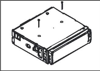
3. Remove chassis from the mounting sleeve.
